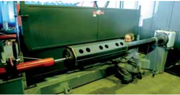
A 1 m long octagonal mast section on a robotic welding station at Hydrospeex in the Netherlands
